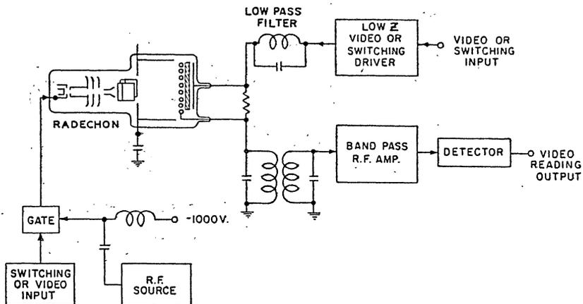
Fig. 4—Radio-frequency signal separation system.
