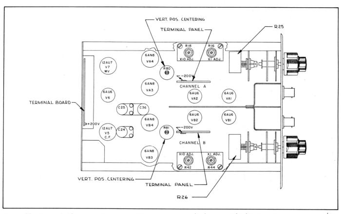
Figure 22. Internal Adjustment Controls and Tube Layout, WB/DI/11 or WB/DI/11-D Dual Trace Preamplifier
