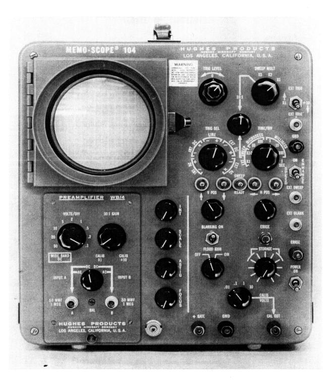
Figure 1. Front Panel, MEMO-SCOPE Oscilloscope, Model 104-D, with WB/4 Preamplifier, Optional Camera Mount, and Speed Enhancement Circuit
