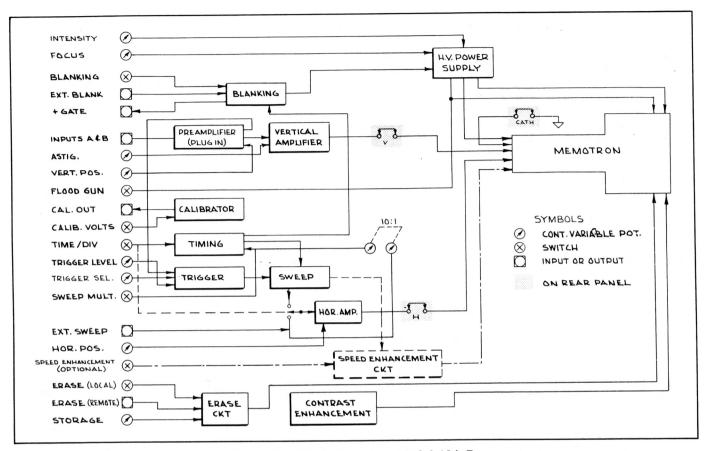
Figure 3. Block Diagram, Model 104-D
