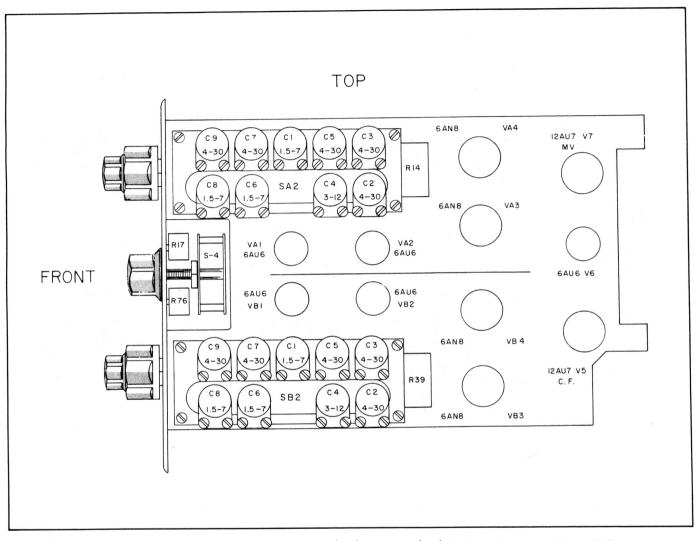
Figure 21. Controls and Tube Layout, WB/DI/11 or WB/DI/11-D Dual Trace Preamplifier
