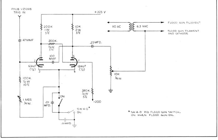
Figure 14. Schematic, Speed Enhancement Circuit
