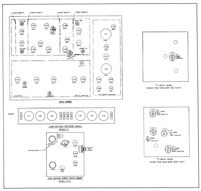
Figure 12. Tube, Potentiometer, and Trimmer Layout, Model 104D
