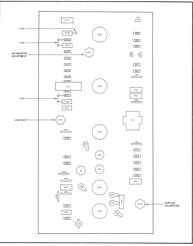
Calibrate Voltage, Storage Circuit, and Vertical Amplifer Location of Parts
