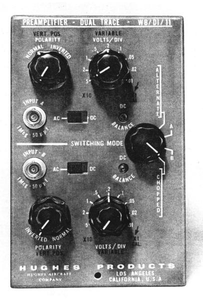
Figure 18. Front Panel, WB/DI/11 or WB/DI/11-D Dual Trace Preamplifier
