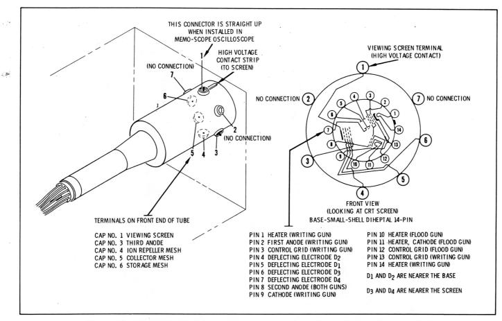
Figure 13. MEMOTRON Tube Pin Locations, and Position of Pins when Installed in MEMO-SCOPE Oscilloscope Chassis
