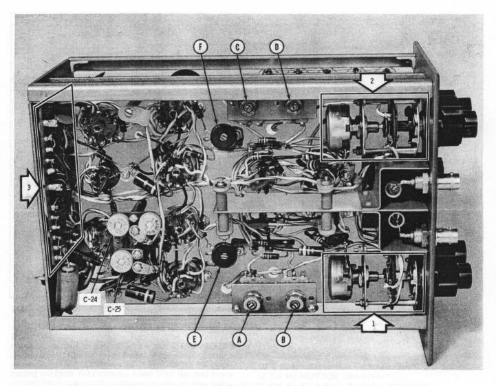
Figure 24. Left-Hand Side View, WB/DI/11 or WB/DI/11-D Dual Trace Preamplifier KEY TO FIGURE 24:
