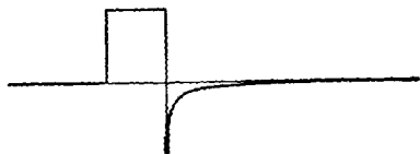
FIG. 3-25.—Spike often produced by shunt capacity.
