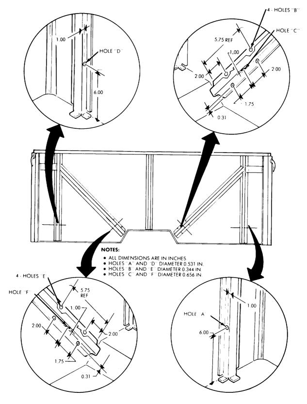
Figure B-1. Cab and Cab Channel Holes
