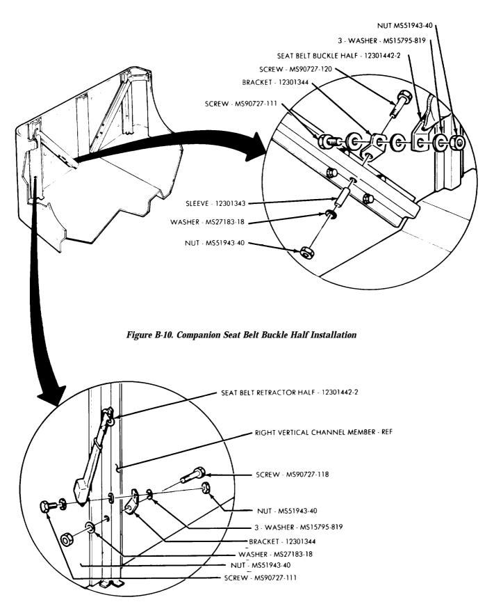
Figure B-11. Companion Seat Belt Retractor Installation
