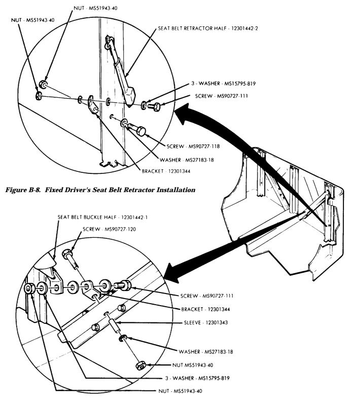
Figure B-9. Fixed Driver's Seat Belt Buckle Half Installation
