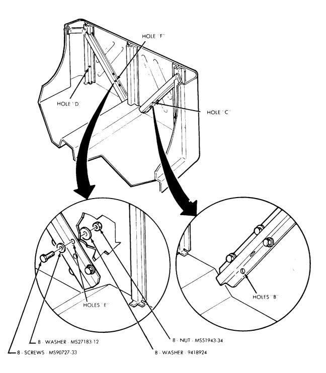
Figure B-2. Cab Channel Reinforcement
