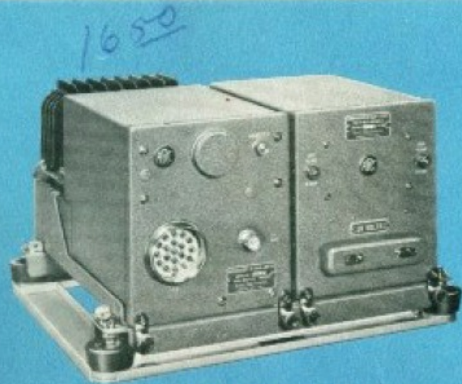
R-34A RECEIVER with DYNAVERTER and B-13A-1 CONVERTER on E-14 RACK AND M-10 MOUNTING
