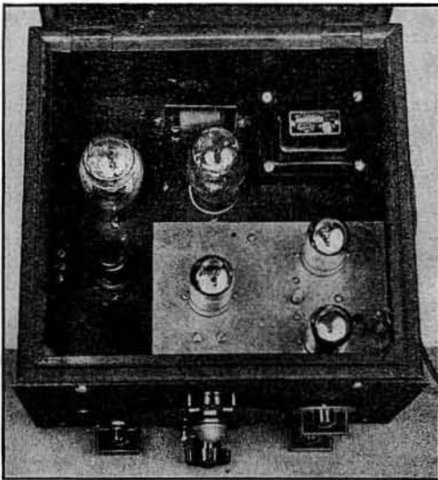
Fig. 1624 — A superregenerative superheterodyne receiver, designed for greater selectivity than can be obtained from the ordinary superregenerator. The audio section is along the left edge of the chassis and the self-contained power supply is at the upper right. The cabinet is approximately 9\frac{1}{2} inches square and 7 inches deep.
