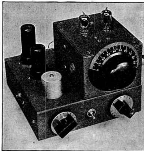
Fig. 1417 — Left — The 112-Mc. r.f. superregenerative receiver uses a 9001 in the r.f. stage, 9002 detector, 6J5 first audio, and 6F6 output stage. The knobs along the front are audio volume control (left) and the regeneration control. The rubber grommet on the side of the 3 \times 4 \times 5 -inch box centers the screwdriver used for setting the detector band-set condenser; a similar one is provided on the other side for the r.f. band-set adjustment. Note the 'phone jack on the side; the speaker terminals are located at the rear. Right — A view under the chassis of the r.f. receiver shows the audio transformer and the arrangement of some of the other components. The three wires coming through the chassis to the right of the "B" + switch are the leads from the r.f. section of the receiver.
