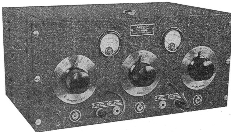
The assembled Lafayette 30-watt transmitter using the 2B6 and 46 tubes.
