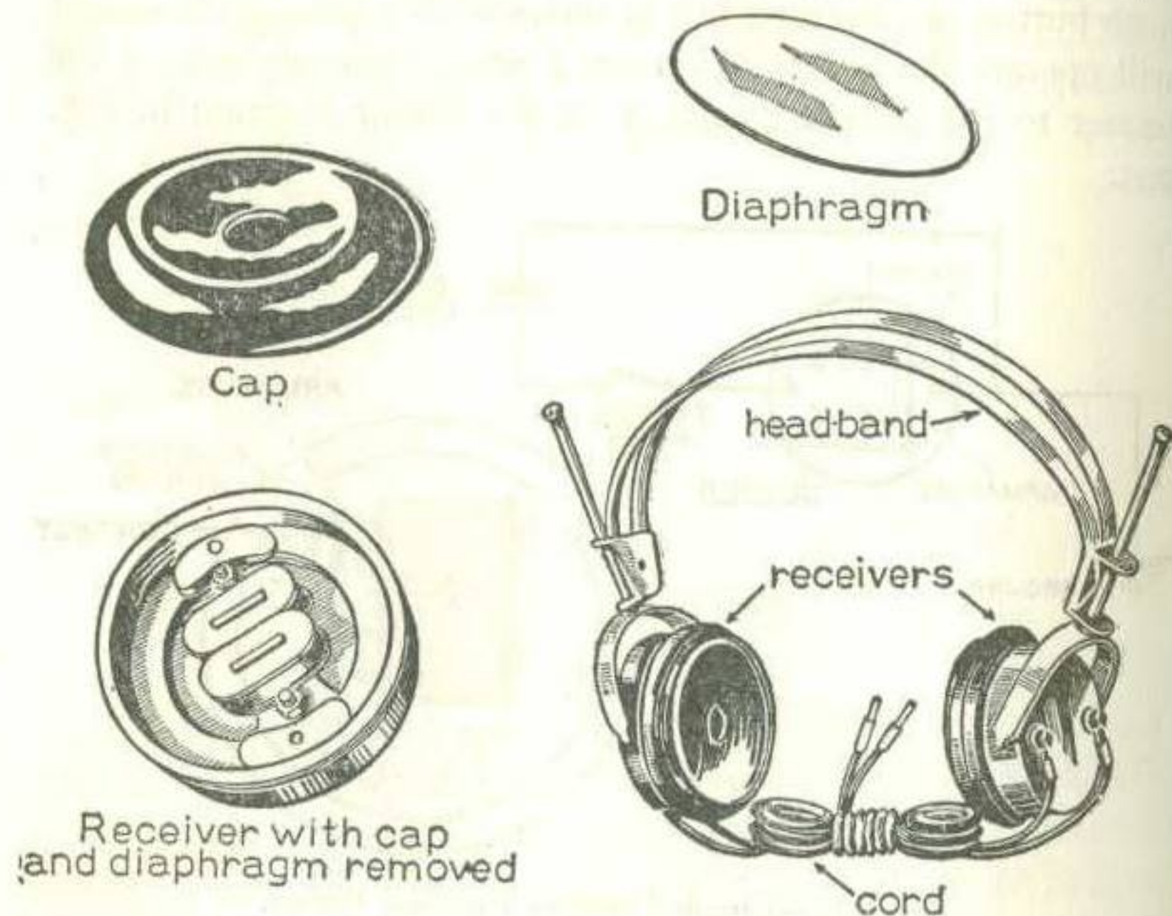
FIG. 202.—A Radio Headset Consists of two Watchcase Type Telephone Receivers Wound with Many Turns of Small-diameter Wire and Mounted on a Headband.
