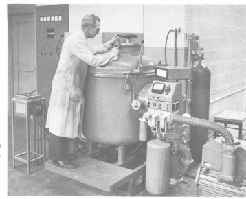
Engineering Laboratory— Experimental vacuum melting furnace.
