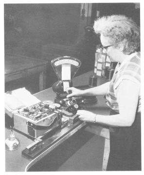
Inspection and Testing of Fine Wire.
