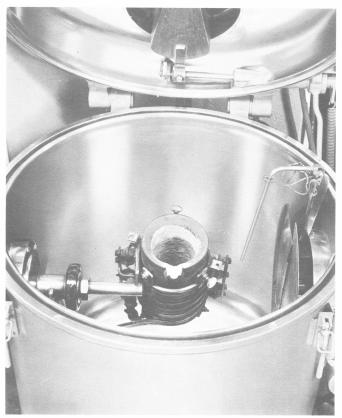
Engineering Laboratory— Inside of vacuum melting furnace.
