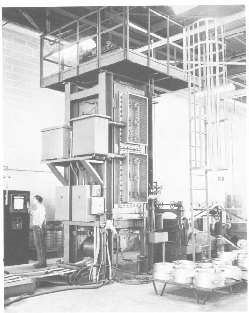
Electric Furnace for Strand Annealing cold rolled strip.
