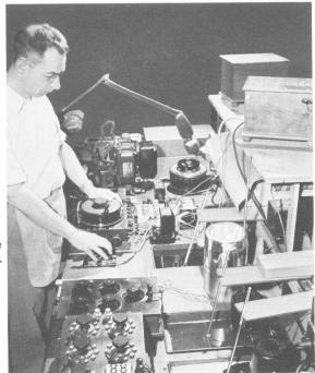
Testing for Temperature Coefficient of Resistance.
