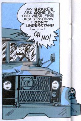
That little piece of cork that goes on the rear wheel drums of these trucks may not look important, but it is. It keeps oil from washing grease out of the wheel bearings. Without grease, the bearings burn up. The oil will get on the brake drum, the lining and the brake shoes.
