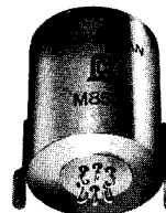
Fig. BB: HERMETICALLY SEALED to meet MIL-T-27. Triple mu metal case, high compression glass terminals, 6-32 x 3/8" mounting studs on 1 1/2" centers; 1" dia. cut out for terminals. Weight: 5 oz.
